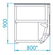
\* at the front with bumpers, the depth of the device is 815 mm
